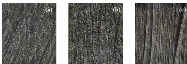
Figure 4 – Micrographs (x50) of the carbon steel surface after 24 hours of immersion in 1.0 mol·dm -3 HCl solution: before immersion (a), in the absence (b) and in the presence (c) of aqueous extract of R. nigrum leaves at a concentration of 1,0 g·dm -3
